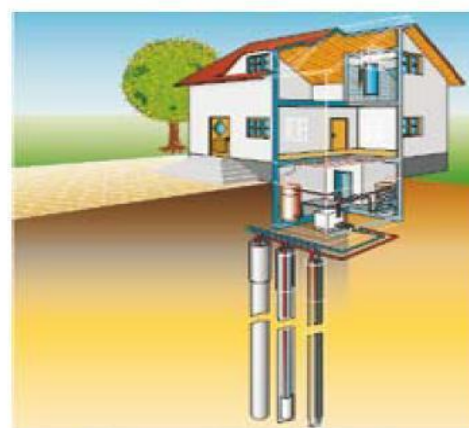
Schema colectori verticali sol
